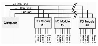
Fig. 12 The controller relies on a high-speed synchronous ring network topology where several remote input/output network nodes (shown as I/O Module #1) collect local sensor data and distribute local actuation commands
