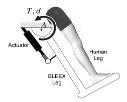
Fig. 2 Simple 1-DOF exoskeleton leg interacting with the pilot leg. The exoskeleton leg has an actuator that produces a torque T about the pivot point A. The total equivalent torque associated with all forces and torques from the pilot on the exoskeleton is represented by d.
