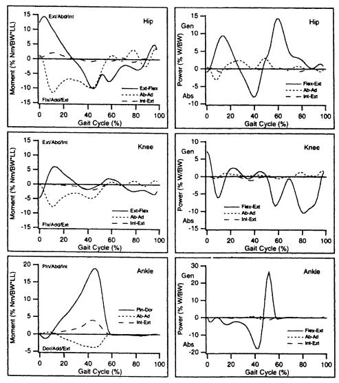
Fig. 15 Human power required for walking. The flexion/extension direction requires the most power for all three joints (ankle, knee, and hip). Besides these sagittal plane directions, the hip abduction/adduction requires the next most power [31].
